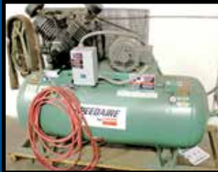
DAYTON SPEEDAIRE 10 HP RECIPROCATING TYPE AIR COMPRESSOR
