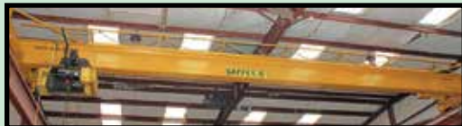
10 T. X 42' SPAN X 64' LONG GANTRY CRANE SYSTEM
