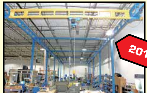
GORBEL 4,000-LB. CAP. FREE STANDING BRIDGE CRANE SYSTEM
