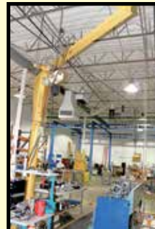
CUSTOM 2 T. CAP. PEDESTAL JIB CRANE
