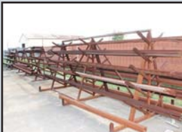
A-FRAME RACK WITH FLAT BAR AND CONTENTS
