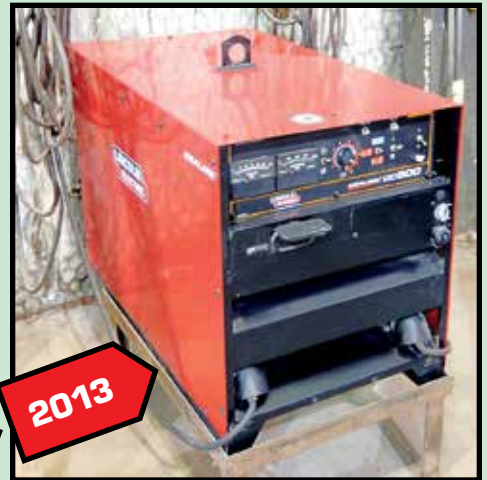
LINCOLN DC600 WELDING POWER SUPPLY
