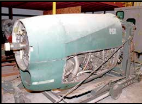
SAMPLE VIEW OF T56 ENGINE CORES
