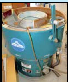
SWECO FINISHING MILL
