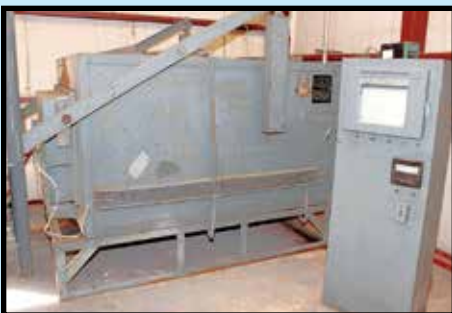
COOLEY HEAT TREAT FURNACE
