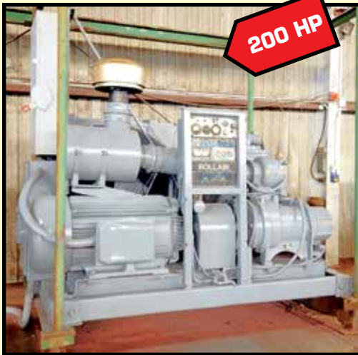
WORTHINGTON ROTARY SCREW AIR COMPRESSOR
