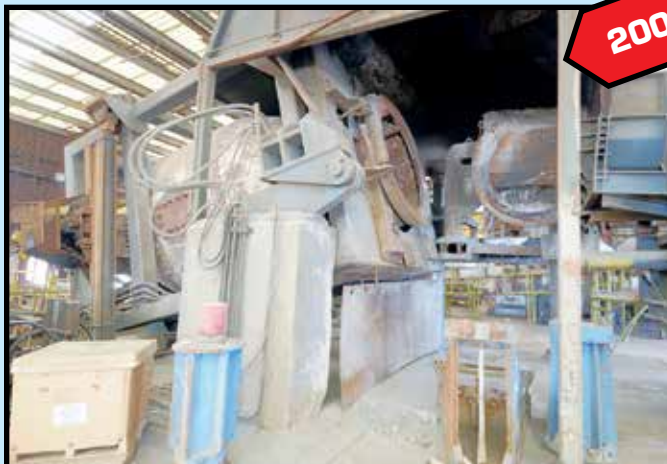
MDY ENGINEERING CORPORATION ROTARY HEARTH FURNACE
