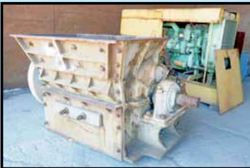
AMERICAN PULVERIZER SHREDDER AND DIESEL GENERATOR
