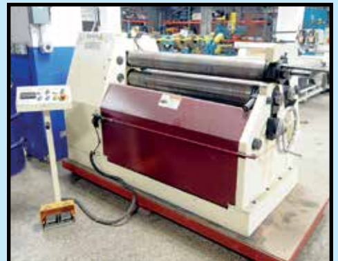
G.M.C. 4' X 1/4" INITIAL PINCH PLATE ROLL
