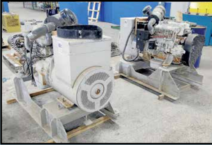
MARATHON 50 KVA DIESEL GENERATORS
