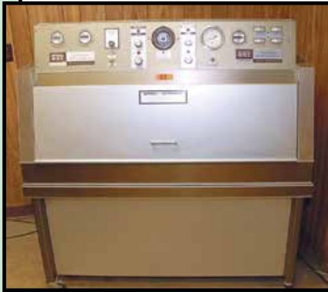
Q-PANEL MDL. QUV ACCELERATED WEATHER TESTER
